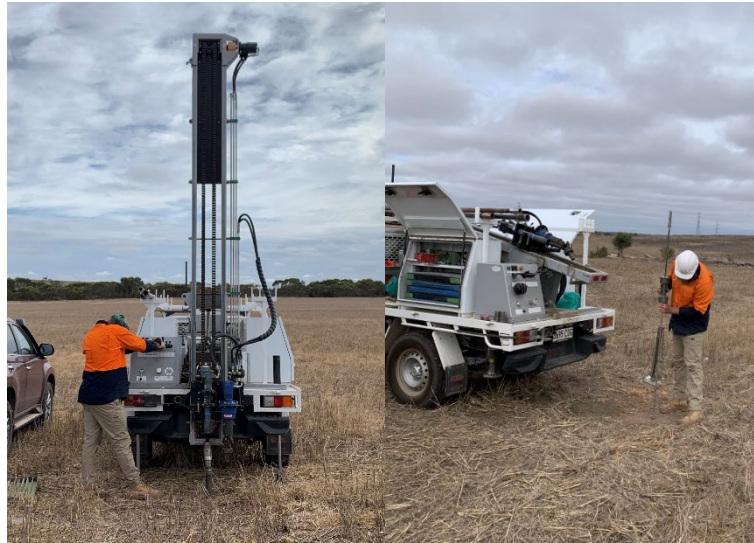
Images: Geotech core sampling works at Riverbend Energy Hub site near Taillem Bend
